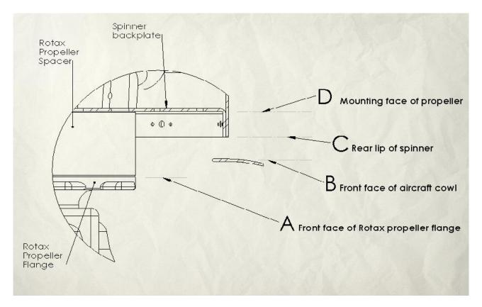
In this case the front of the engine cowl (B) is forward of the front face of the Rotax propeller mounting flange (A). Clearly a spacer is required to move the propeller / spinner forward but it must be decided how much this should be.
